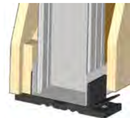
Vibro-WS support systems for a floating gypsum board partition
